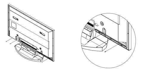
2 Set the Speaker Guide Bracket into the square grooves located on either side of the PDP's bottom rear, then push the Speaker Guide Bracket towards the center (as the arrow illustrates). Secure the Speaker Guide Bracket with provided screws (2). (Always use the proper screws, as indicated.)
